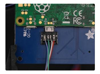
Connect USB OTG Adapter Before mounting the components, go ahead and plug in the micro USB OTG adapter to the Raspberry Pi.
