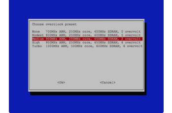
You can access the **raspi-config** utility from the RetroPie configuration screen, or press "F4" to exit to a command line and run "sudo raspi-config" manually.
